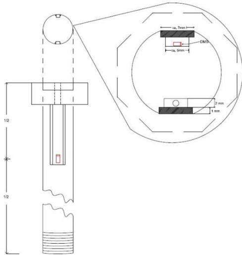
Fig. 2: Modified Bolt
