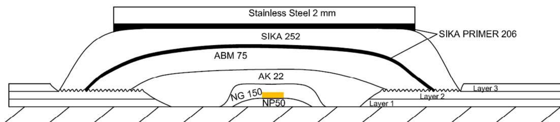
Fig. 1: Application of strain gauges
