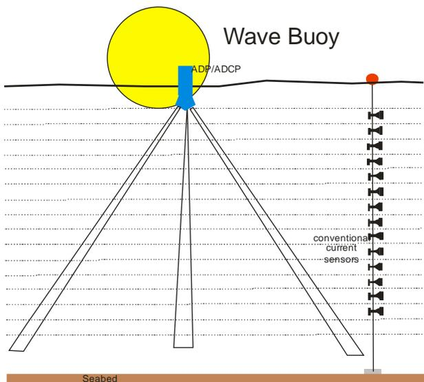
Fig.6: Buoy hull with integrated ADCP/ADP
